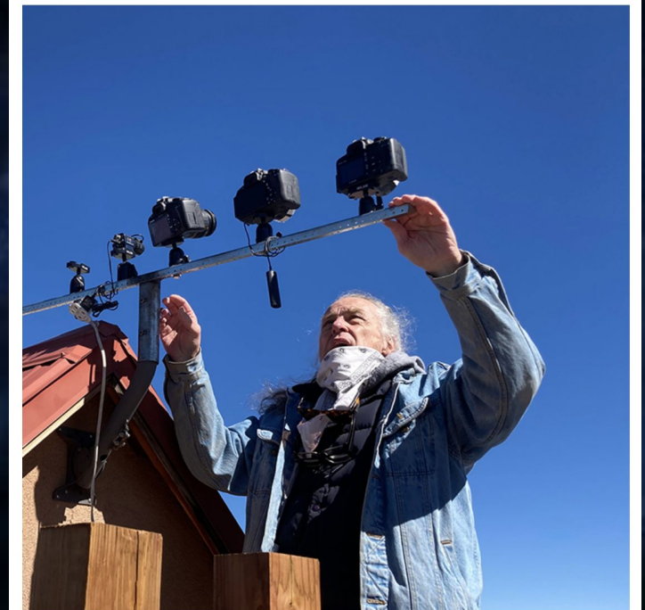
Thomas prepares his purpose-built camera array for capturing images of “jellyfish sprites.” Sprites are brief, colorful flashes of light sometimes seen high above thunderstorms. . Image credit: Lynn Larsen
