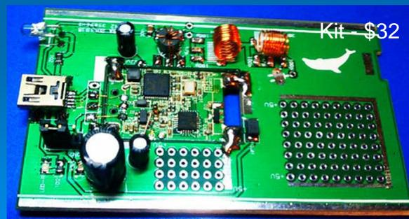
Inexpensive options are available to obtain HF coverage with the basic RTL-SDR. A separate upconverter that can be added in front of a standard RTL-SDR for about \$40, although putting it in a well shielded metal box is recommended and adds a few more dollars to the price.
