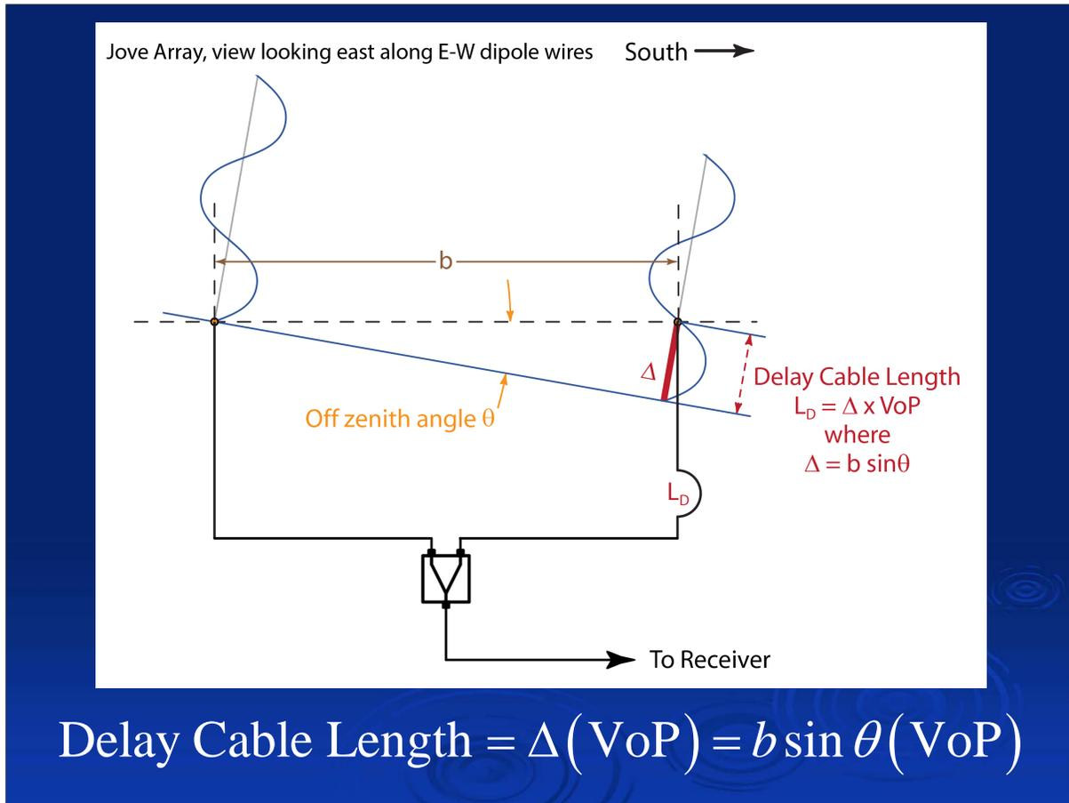
Here is an example of a simple phased array, the Jove array.
