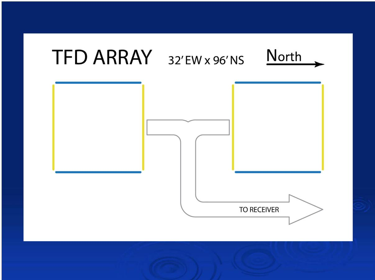
Since the TFD array is a combination of the yellow and blue portions, simple beam steering, however, does not tell the whole story! To see where the beam of the whole array is pointing, we have to analyze the pattern of a TFD element, the pattern formed by an array, and the combinations they form.
