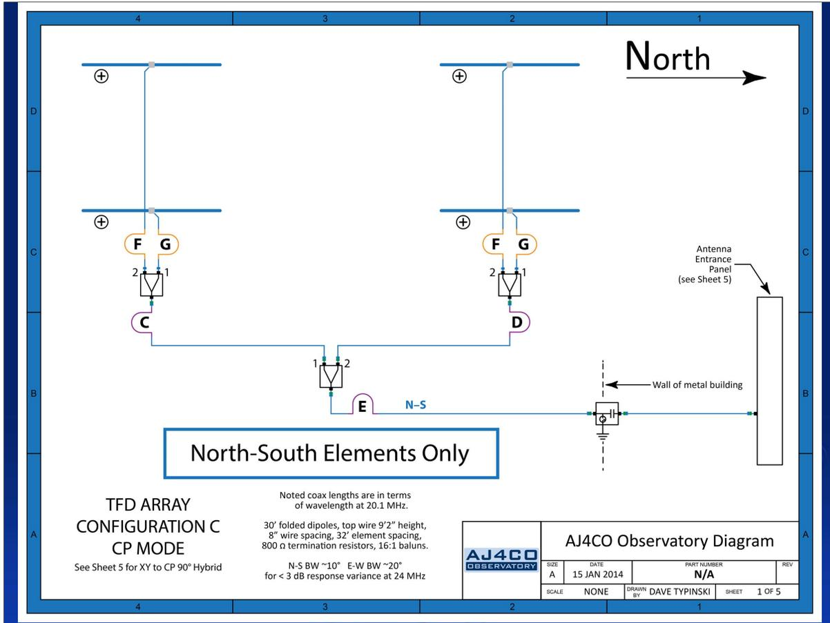
The other is all the north-south elements. This diagram shows the associated delay cable positions. Varying the length of the ORANGE delay cables steers the beam east and west. Varying the length of the PURPLE delay cables steers the beam north and south.
