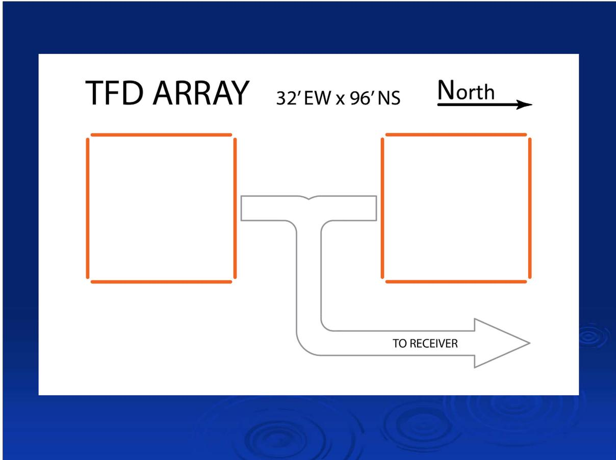
Here is a diagram of the 8-element TFD array. Two squares, each 32 by 32 feet, separated from each other by 32 feet.
