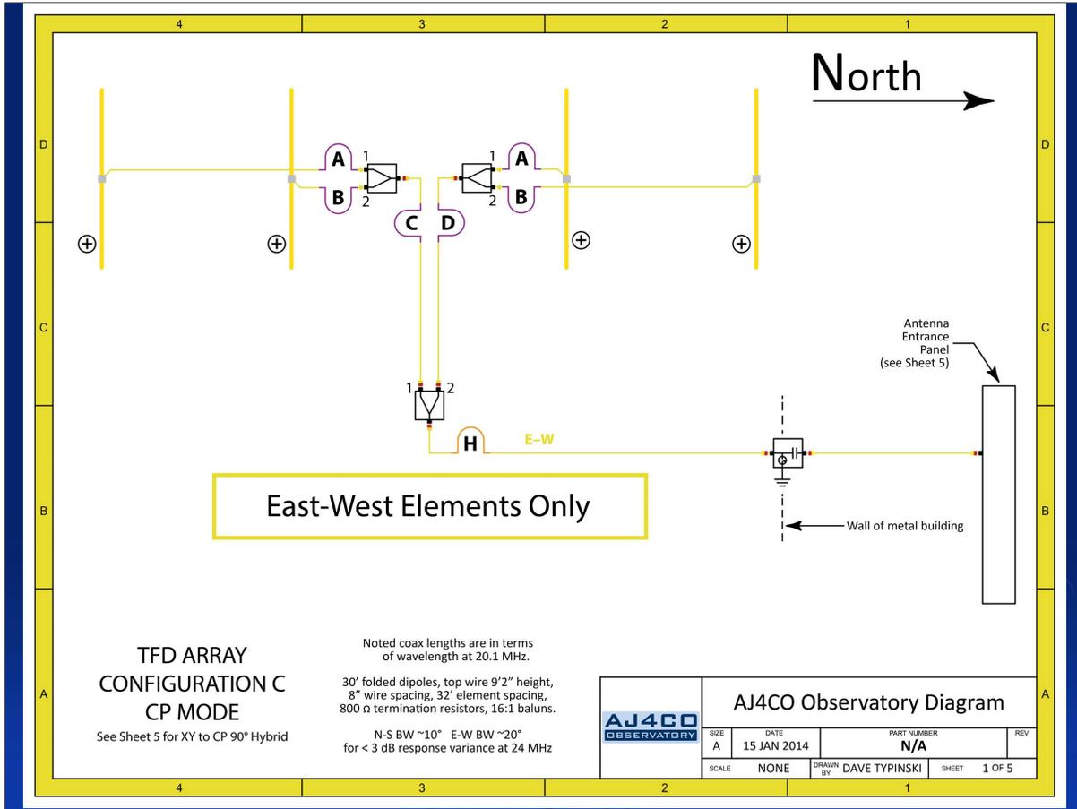
The TFD array is really a combination of two arrays. This is one: all the east-west elements. This diagram shows the associated delay cable positions. Varying the length of these delay cables steers the beam north and south.
