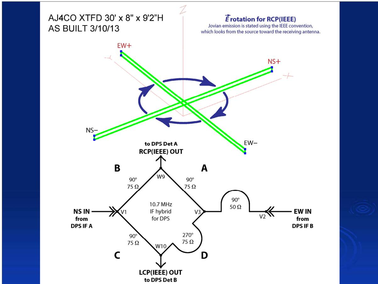
The DPS doesn't *have* to be used for RCP and LCP – it can accept any two RF inputs and record correlated samples. We have used RCP and LCP because that seems the most useful option.
