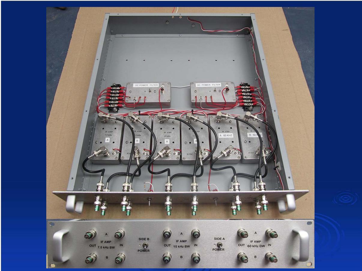
Here is a picture of the DPS auxiliary IF strip chassis. There are three pairs of aux IF strips, one for each side of the DPS at 7.5, 15, and 60 kHz bandwidth. The two 30 kHz wide IF strips are in the main DPS unit.
