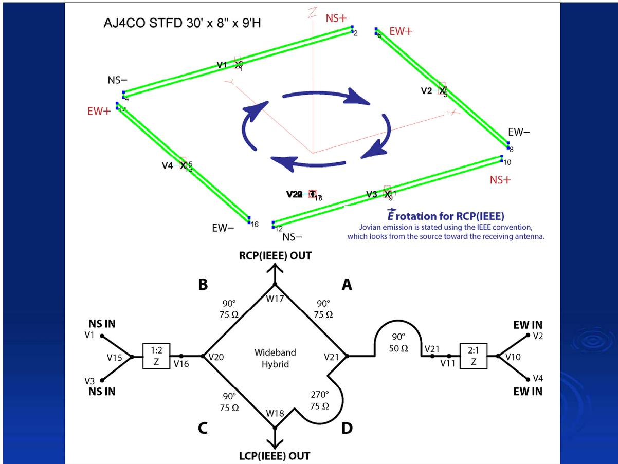
One “square” of the TFD array. A square is just an expanded cross (slide #9); the separation of RCP and LCP works the same. The curved arrows in the diagram only show the rotation of the emission’s electric field vector for RCP; they do **NOT** show the instantaneous polarity of each element in the square array. For example, when the E vector is pointing east, **BOTH** east-west elements see the E vector pointing east – that is, they see the same signal, in phase.
