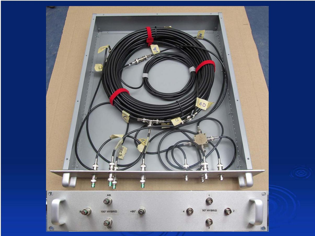
**Rear:** DPS 10.7 MHz 180° hybrid ring made from 112 feet of RG-6 75 ohm coax. The letters on the masking tape labels correspond to the lettering of the wire segments shown on slides that follow. The small inner ring is a 90° RG-58 50 ohm coax phase delay cable that precedes one of the larger ring's inputs (as shown on the same slides). Connection of the narrowband 10.7 MHz hybrid is discussed on slides that follow.
