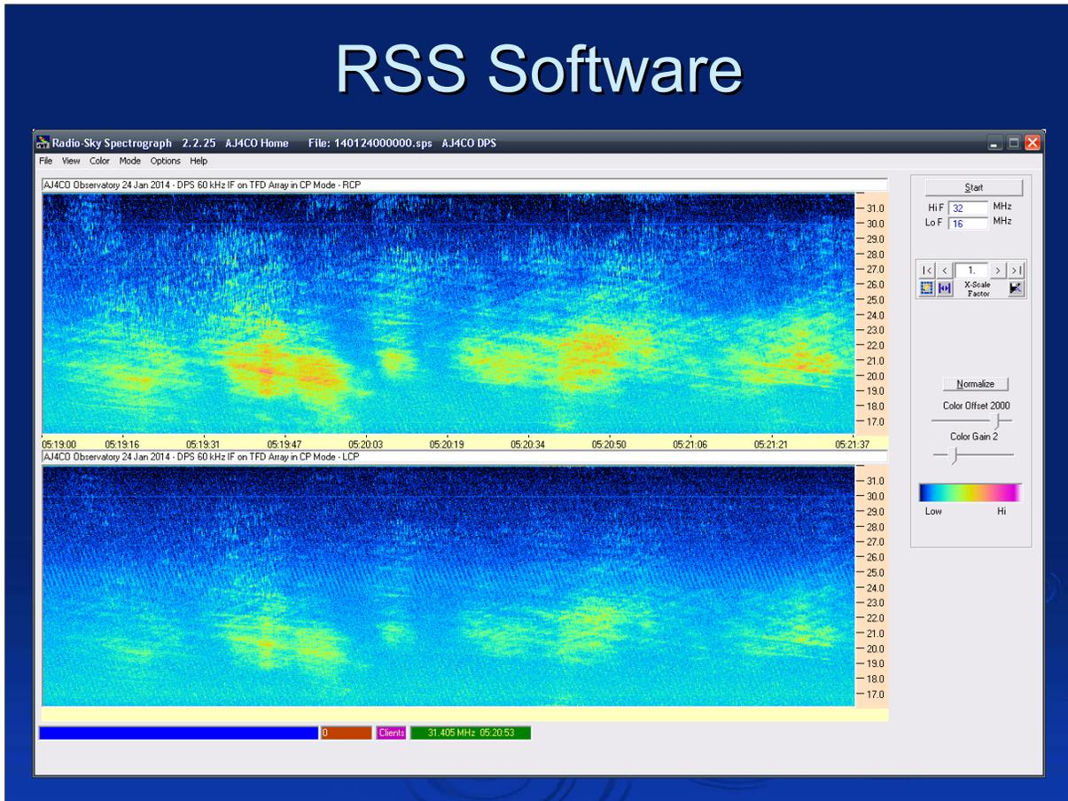
The DPS hardware is controlled by the Radio Sky Spectrograph (RSS) software. Jim Sky, who graciously makes RSS available to all for free, made several modifications to RSS to allow it to control the DPS, record two correlated spectral data streams, and display two waterfalls in real time.
