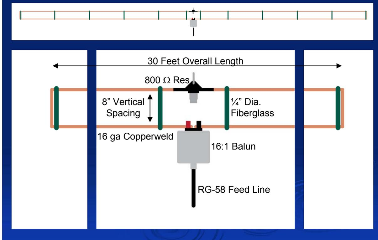
A diagram of a terminated folded dipole (TFD) element.
