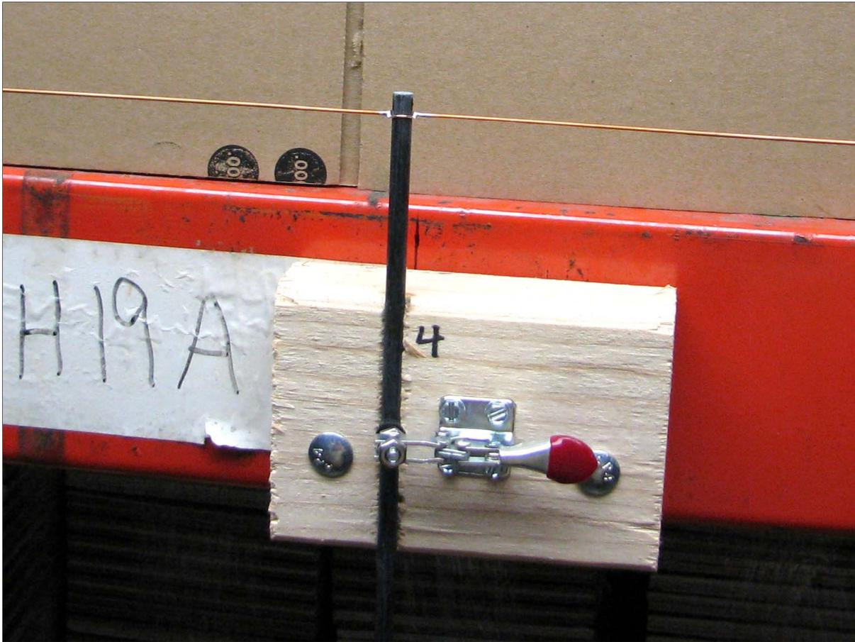
The 16 ga Copperweld element wires have an 8" spacing maintained by cross-drilled fiberglass rods. A short U-shaped loop of 22 ga copper is soldered around the rod to keep the rod from sliding along the Copperweld. This is one of a series of six toggle clamps used to position the rods during element construction.
