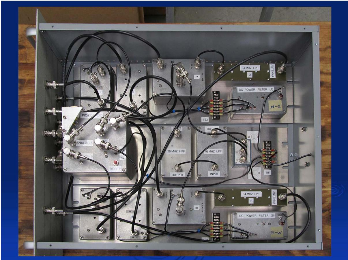
The three DPS blocks shown in the previous diagram installed in a 19" chassis.
