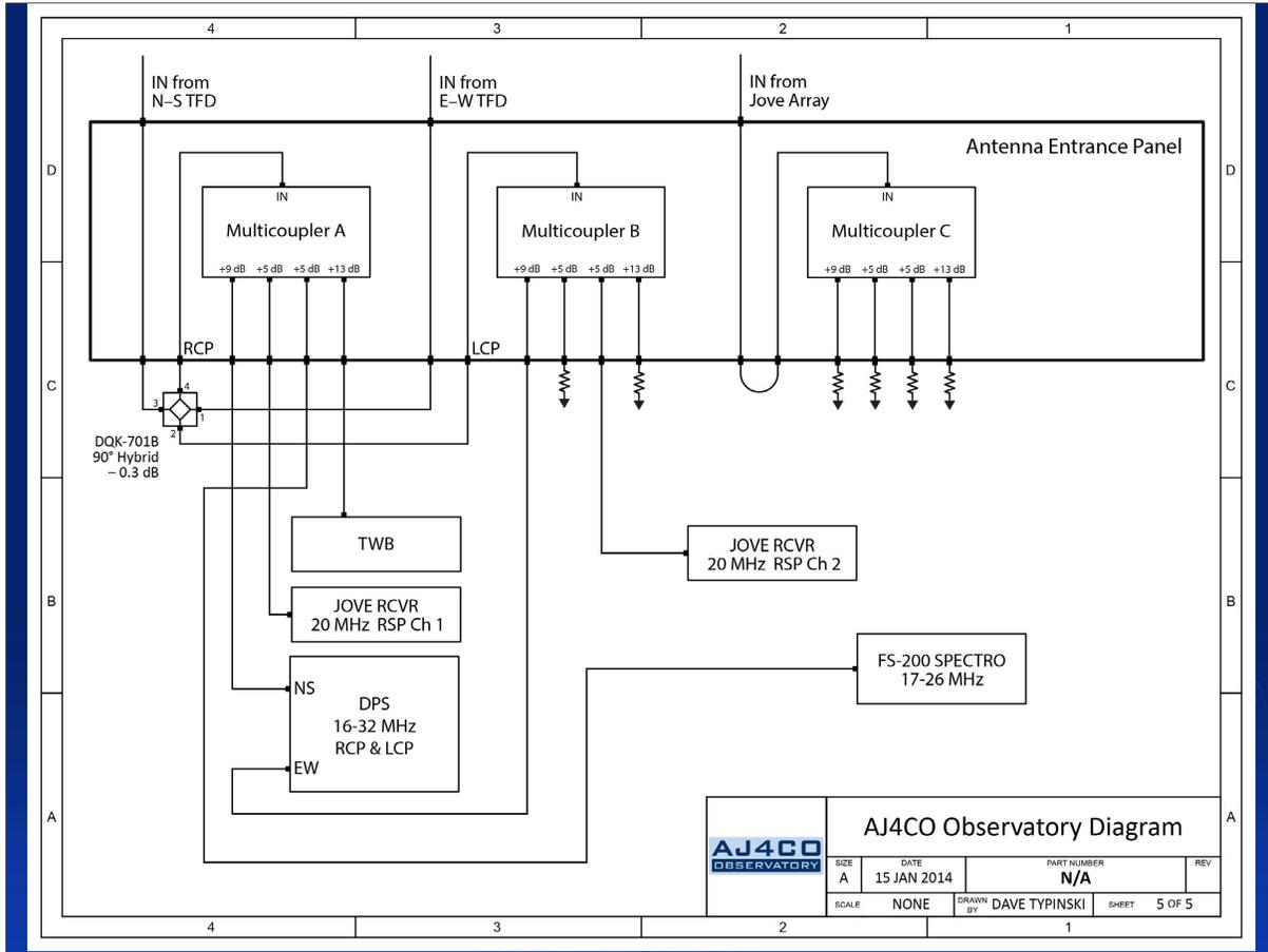
Shown here is the observatory antenna connection and signal distribution schematic.
