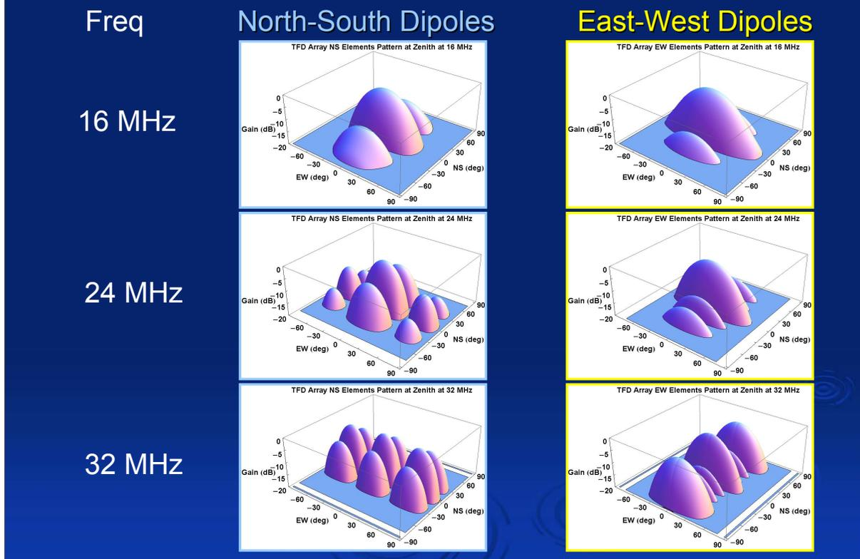
And here are the real beams (array steered to zenith), found by simply multiplying the array factors by the element Factors. This is **much** easier than running the electromagnetic field calculations for eight real TFD antennas spaced 32 feet apart in a rectangular array.
