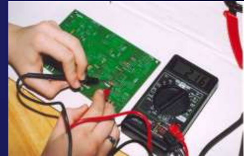
Checking resistor with multi-meter
