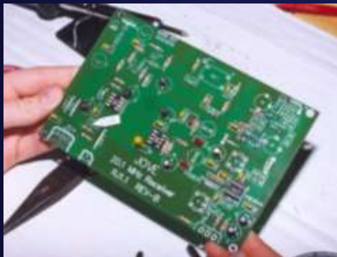
Inspecting solder connections
