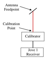
You must know cable type and length, or loss (in dB), from the antenna. feedpoint to the calibration point.
