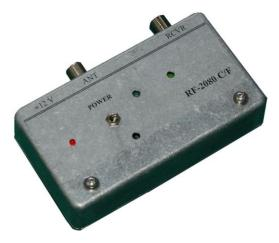
A single toggle switch controls power and also selects the source of the signal being routed to the receiver (noise source or antenna).
