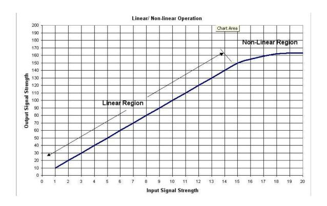
In the linear region we can calibrate the system at a single point. Calibration means measuring the SPU for a known noise temperature at the receiver antenna terminals. A simple equation relates SPU to temperature for all other signals in the linear region. However, if signals go into compression then the calibration is no longer valid.
