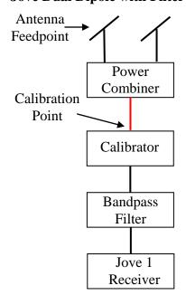
Calibrator installed between antenna and filter. Cal Wizard will supply loss data from antenna feedpoint to power combiner output.
