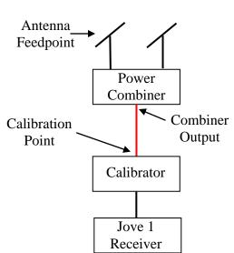
You must know cable type and length, or loss (in dB), from calibration point to power combiner output. Cal Wizard will supply loss data from the antenna feedpoint to the power combiner output.
