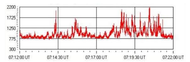
The horizontal axis is time while the vertical axis is in SkyPipe Units (SPU). For this record the receiver and software gain controls were set so that the baseline runs around 800 units on the vertical scale with the strongest burst extending up to 2200 units.
