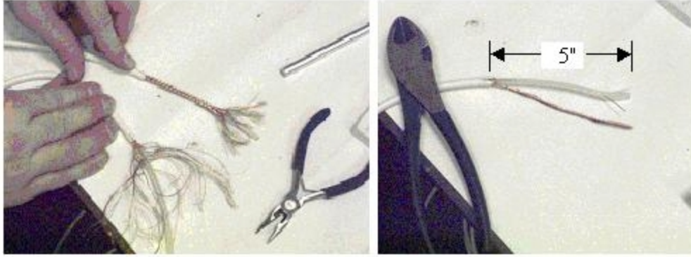
Figure 3a and 3b. Unbraid and twist copper shielding.
