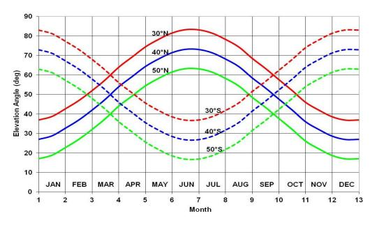
Figure 1.1. Shown is the maximum elevation angle of the Sun throughout the year for observers at different latitudes. Solid curves are for northern hemisphere observers (at 30°N, 40°N, and 50°N) and dashed curves are for southern hemisphere observers (at 30°S, 40°S, and 50°S).
