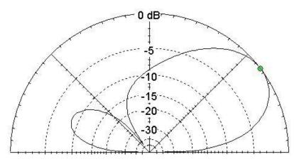
Dual dipole, 20 ft, 90 deg phasing, gain = 9.1 dBi at el = 37
