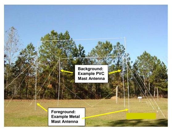
Figure 7.3c. Twenty foot masts comparing PVC and metal.
