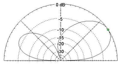
Dual dipole, 20 ft, 135 deg phasing, gain = 9.5 dBi at el = 33
