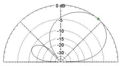
Dual dipole, 15 ft, 90 deg phasing, gain = 8.7 dBi at el = 49
