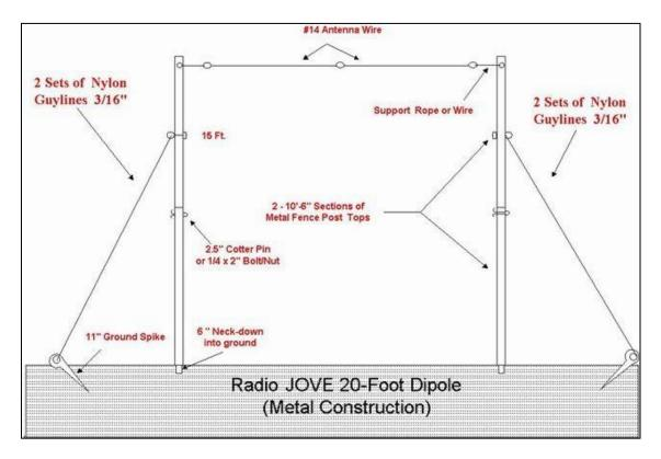
Figure 6.5. Side-view schematic of metal mast dipole installation.
