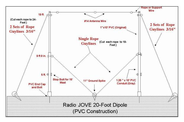
Figure 6.3. Side-view schematic of PVC mast dipole installation.
