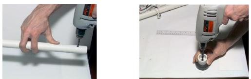
Figures 6.1a and 6.1b. Drill the PVC piping (¼ in. drill bit) and end cap (3/8 in. bit).
