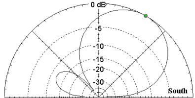
Figure 3.9. A 90° phasing cable added to the south dipole coax steers the antenna beam south. In this example the dipole array is 10ft high and the beam center is approximately 60° above the southern horizon.
