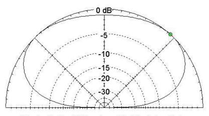
Single dipole, 15 ft, gain = 5.7 dBi at el = 48 deg
