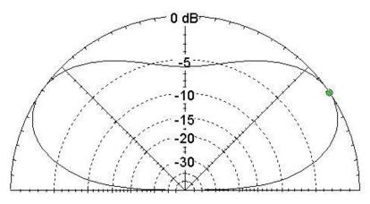
Single dipole, 20 ft, gain = 6.3 dBi at el = 34 deg
