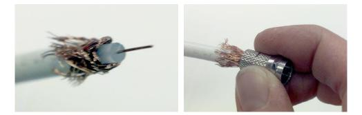
Figure 5.6d – 5.6e. Prepare the coax and install the F-connector.
