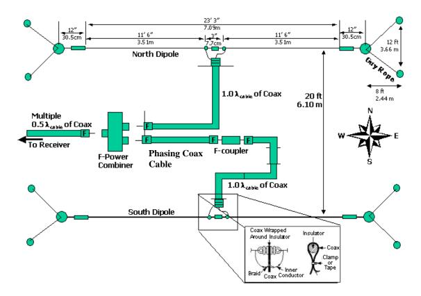
Figure 7.2. Top-view schematic of Radio JOVE dual dipole with phasing cable inserted in the southern dipole feedline. This will steer the beam to the south. For southern hemisphere use the phasing cable will be in the north dipole feedline.
