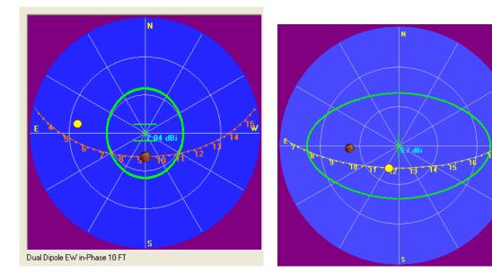
Figure 3.14. RJP plot showing the overhead antenna beam and the track of Jupiter across the sky in July 2011 for a station located at 30°N.
