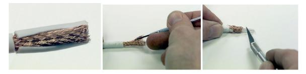
Figure 5.6a – 5.6c. Prepare the coax and install the F-connector.
