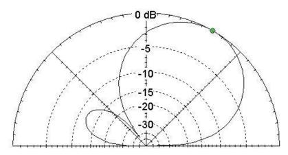
Dual dipole, 10 ft, 90 deg phasing, gain = 8.5 dBi at el = 60
