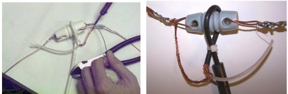
Figure 5.4. Solder the shielding and center conductor to the copper wires. Figure 5.5. Install the ferrite toroid cores.
