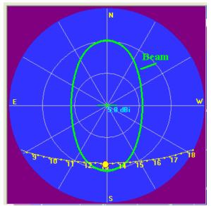
Figure 3.3. The beaming pattern for a single dipole antenna mounted at a height of 10 ft at a station at 30°N. The track of the Sun is for December when it is furthest south. At this time the Sun is in the beam for only 2 hours but throughout the rest of the year when the Sun is further north observing time is longer.
