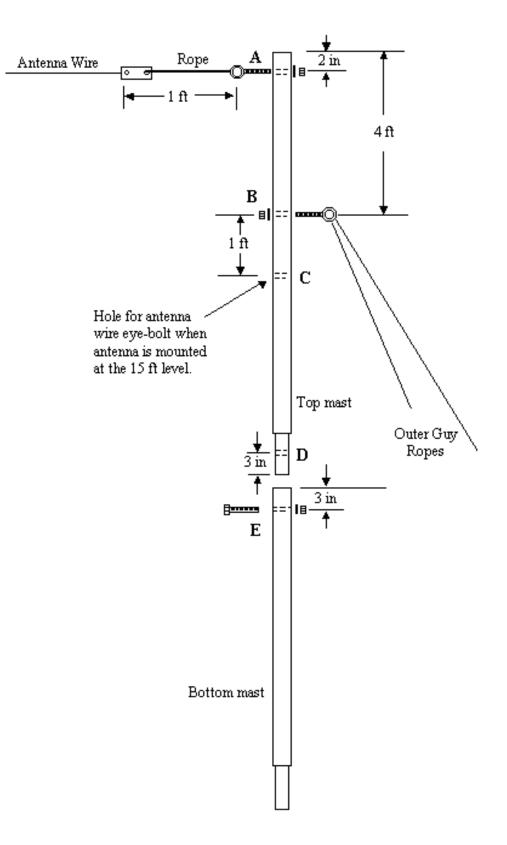
Figure 6.4. Metal Mast Assembly.
