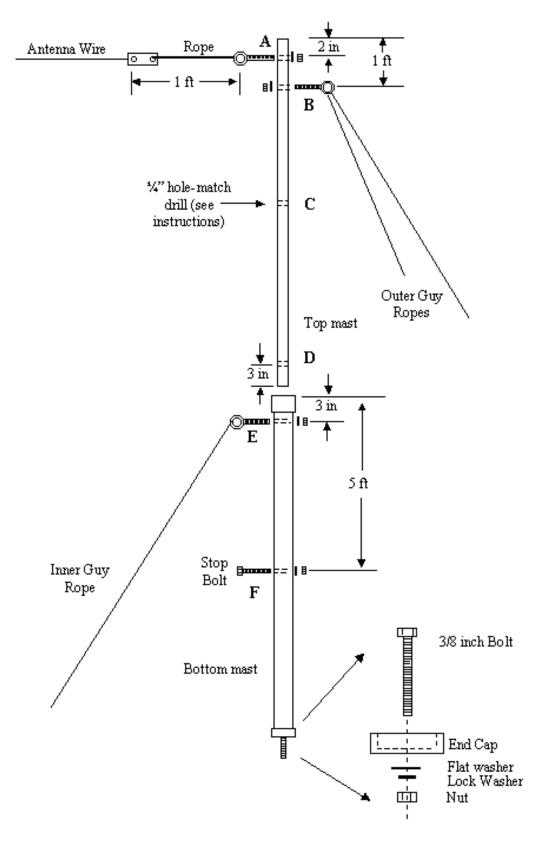
Figure 6.2. PVC Mast Assembly.
