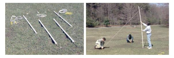
Figure 7.3a and 7.3b. Sample pictures for 10-foot mast setup. Lay out each dipole on the ground and set up one pole at a time.
