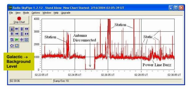
Figure 7.5. Sample RJ output showing a typical SkyPipe record. The effect of connecting and disconnecting the antenna is clearly seen.
