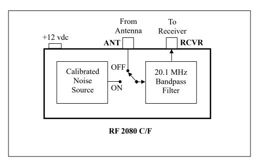
A single toggle switch controls power and also selects the source of the signal being routed to the receiver (either the antenna or the noise source). When the 2080 is OFF the antenna is connected to the receiver. When it is ON the calibrated noise source is connected to the receiver. In the C model the switch common is connected directly to the RCVR connector (a direct connection replaces the bandpass filter).
