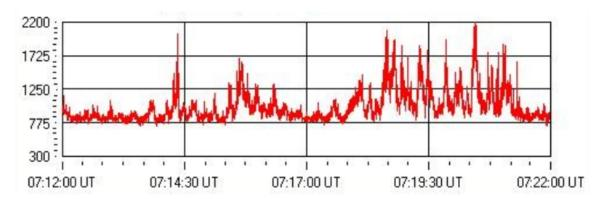
The horizontal axis is time, and the vertical axis is in SkyPipe Units (SPU). For this record the receiver and software gain controls were set so that the baseline runs around 800 units on the vertical scale with the strongest burst extending up to 2200 units.
