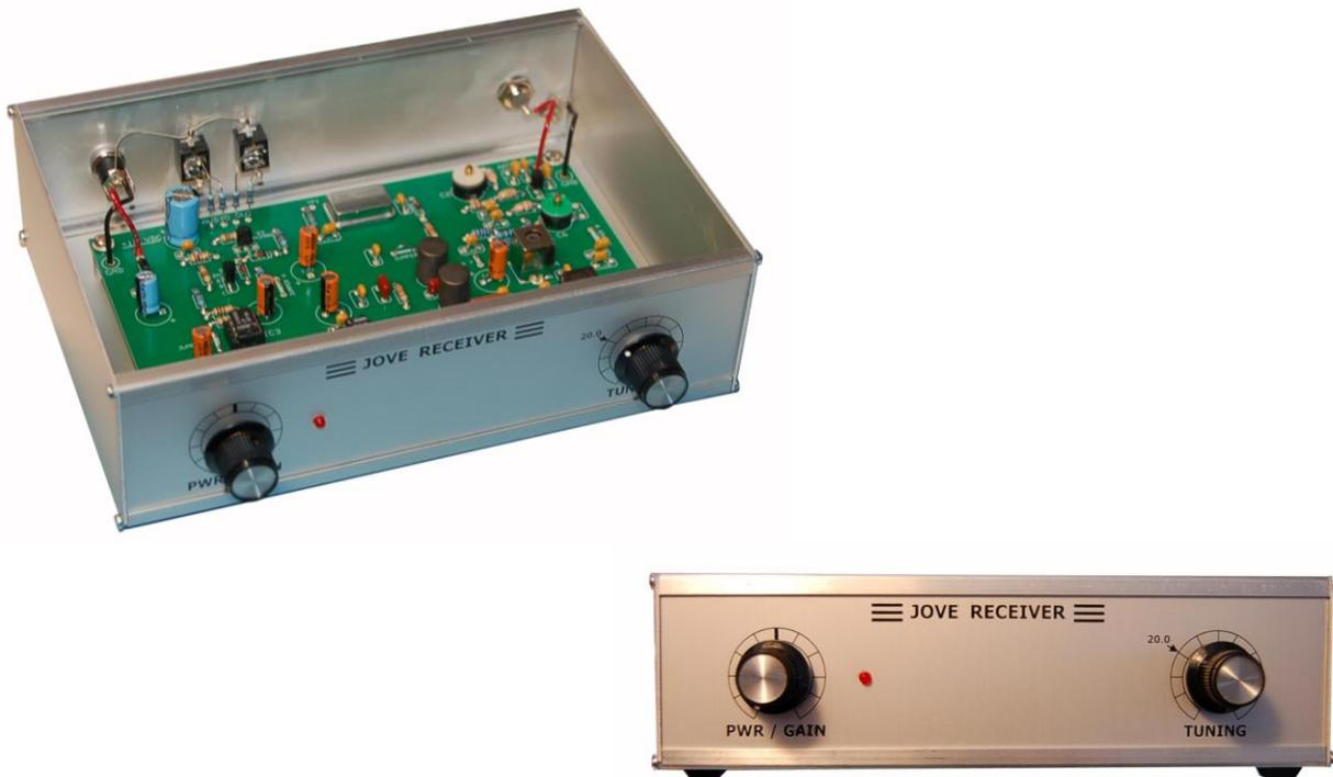
Figure 19. Views of completed JOVE RJ1.1 receiver
