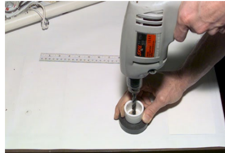
Figures 6.1a and 6.1b. Drill the PVC piping (1/4 in. drill bit) and end cap (3/8 in. bit).
