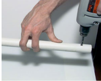
Figures 6.1a and 6.1b. Drill the PVC piping (1/4 in. drill bit) and end cap (3/8 in. bit).
