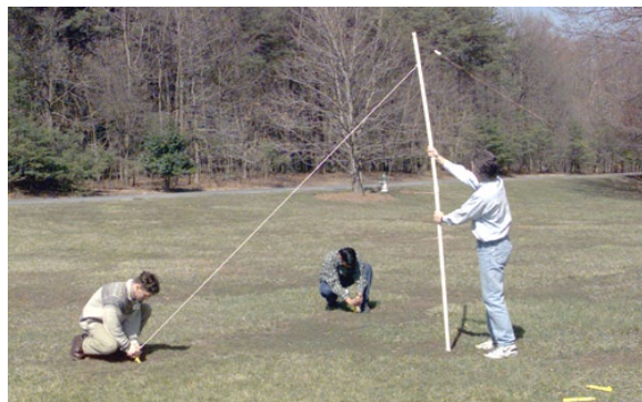
Figure 7.3a and 7.3b – Sample pictures for 10-foot mast setup. Lay out each dipole on the ground and set up one pole at a time.
