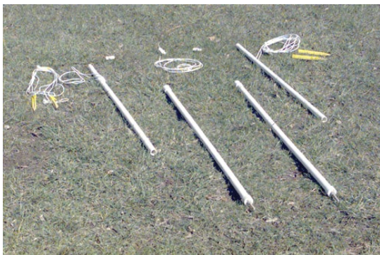
Figure 7.3a and 7.3b – Sample pictures for 10-foot mast setup. Lay out each dipole on the ground and set up one pole at a time.
