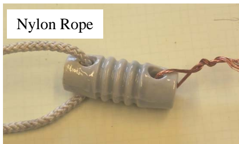
Figure 5.1a and 5.1b. Wrap the center and end insulators with the antenna wire.
