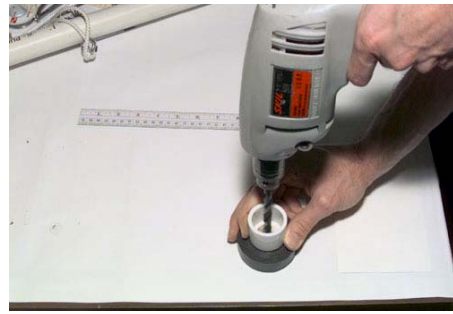
Figures 6.1a and 6.1b. Drill the PVC piping (1/4 in. drill bit) and end cap (3/8 in. bit).
