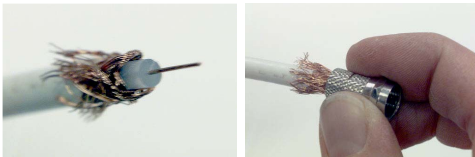
Figure 5.6d – 5.6e. Prepare the coax and install the F-connector.
