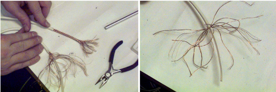
Figure 5.2a and 5.2b. Unbraid the copper shielding.
