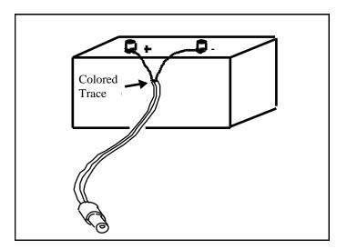
Figure 15. Wiring the power plug to a battery - the colored tracer goes to the + side of the supply.
