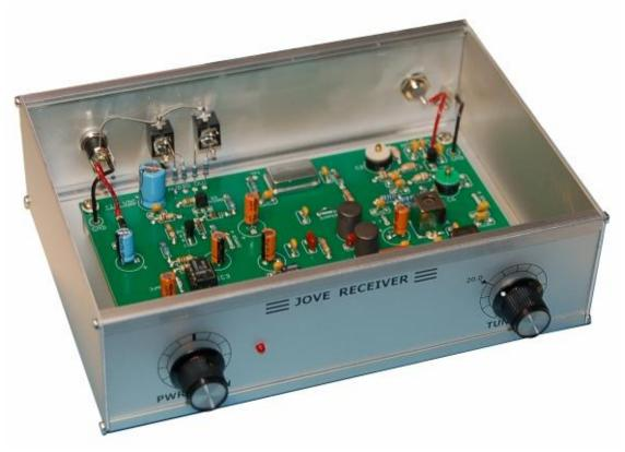
Receiver Kit and Manual developed for NASA JOVE Project by Richard S. Flagg, RF Associates rf@hawaii.rr.com This page intentionally left blank.
