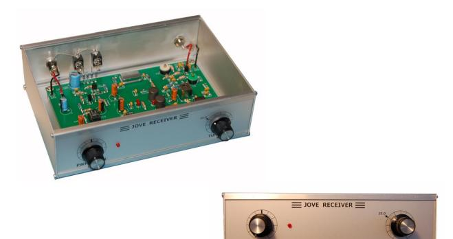
Figure 19. Views of completed JOVE RJ1.1 receiver
