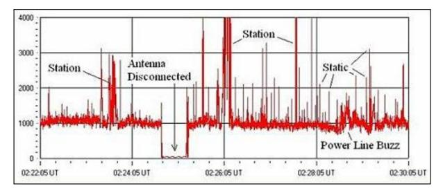
Figure 18. Example Radio Jove output using Radio-Skypipe display software
