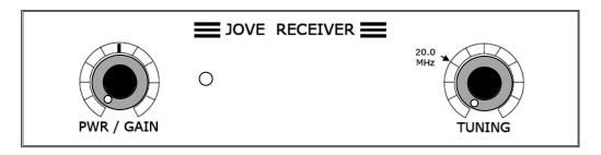
Figure 10. Jove receiver front panel with knob alignment.
