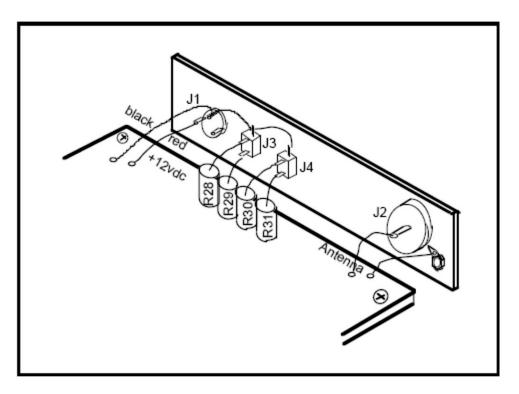
Figure 13. Rear panel wiring (resistor R32 not shown)
