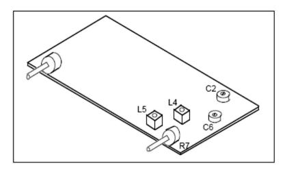
Figure 17. Locations of the variable capacitors and inductors
