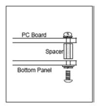
Figure 14. Mounting the spacers to the bottom panel
