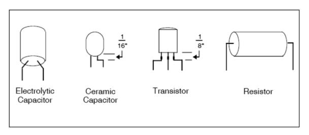
Figure 6. Forming the component leads to match up with PC board hole spacings
