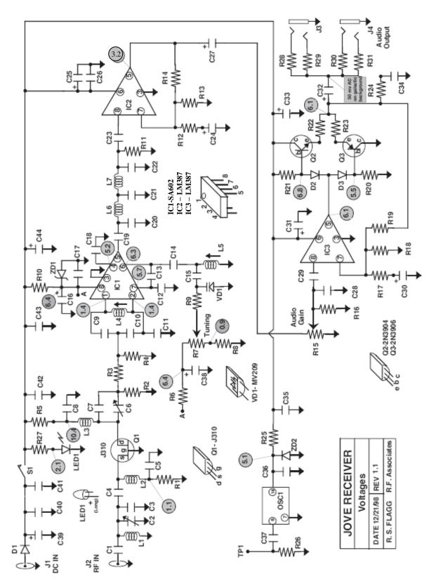
Figure 20. JOVE receiver schematic with DC voltages
