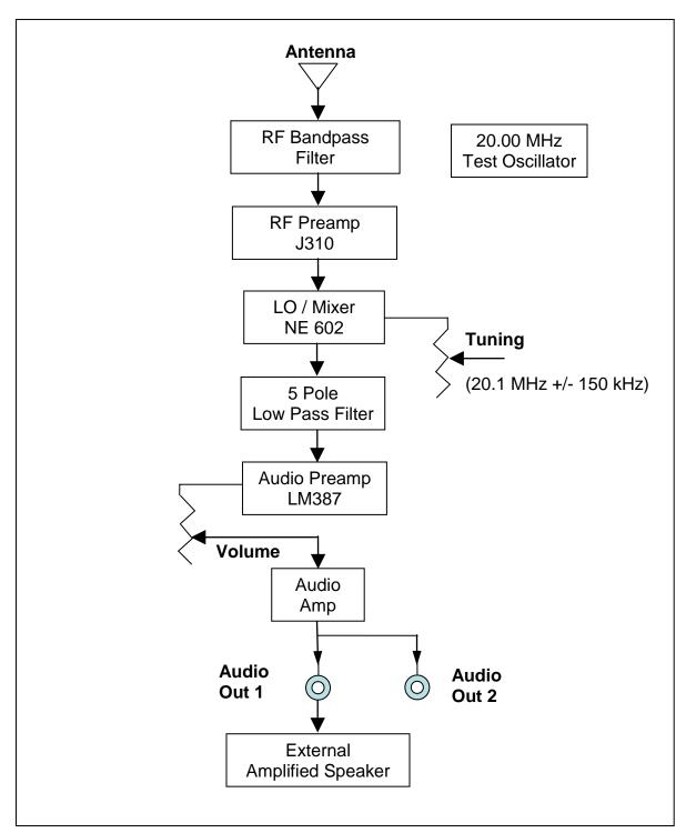
Figure 1. JOVE receiver block diagram
