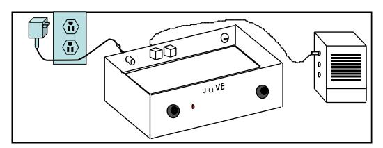
Figure 16. Test set-up, radio with the cover off connected to the AC Adapter and the amplified speaker
