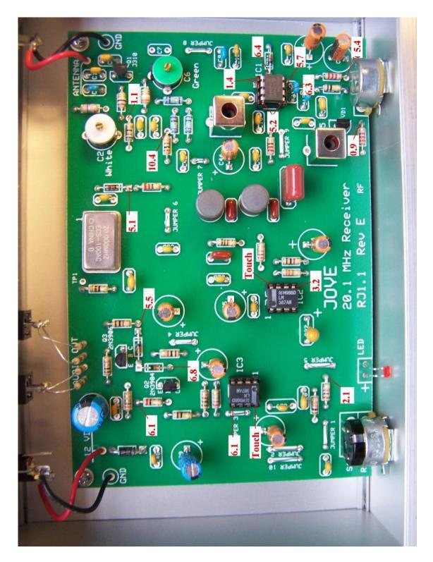
Figure 21. JOVE receiver board with DC voltages for testing
